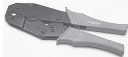
F24-9858P RG-58, RG-59TFE & F24-9859P RG-59, RG-62 Standard Series Ratchet Crimping Tools This series of tools offers a wide selection of interchangeable dies, a high quality steel frame with a full cycle ratchet mechanism and a quick release safety latch. Crimps 2pc. BNC and TNC connectors.
