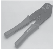
F24-8860P Ratchet Crimping Tool for 3-Piece Crimp Connectors. Offset die with 3 crimp sizes for Pins & Connector Ferrule including RG-58 & 59TFE Cable. Features adjustable crimp pressure and quick release safety latch.
