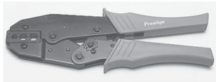
F24-8866P 'F' Ratchet Crimping Tool Crimps RG-59, RG-6, and RG-Quad Shield 'F' type CATV connectors. Features adjustable crimp pressure and quick release safety latch. Hex Sizes: .255", .324", .354"
